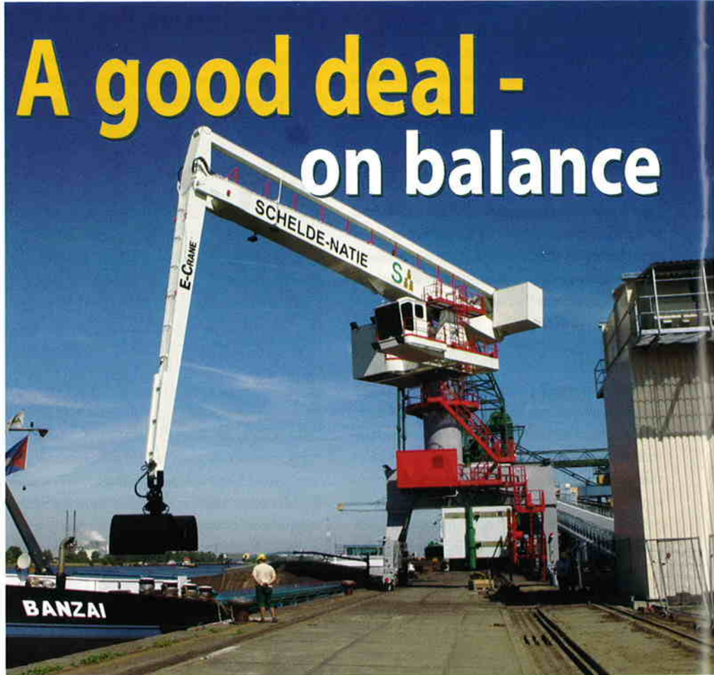
Due to their build simplicity balance cranes offer a much longer lifespan than other cargo handling equipment
